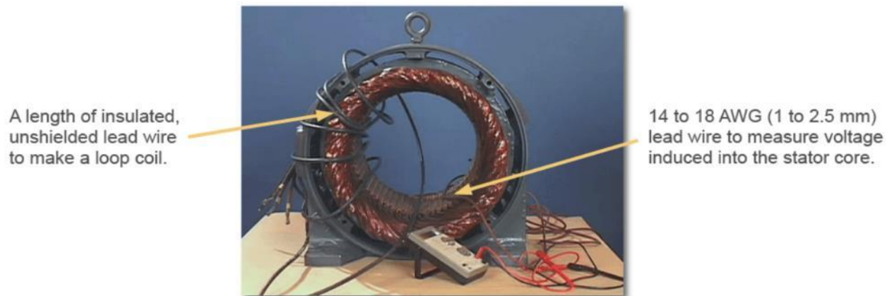
Figure 50: Core loss testing using a non-commercial core tester
