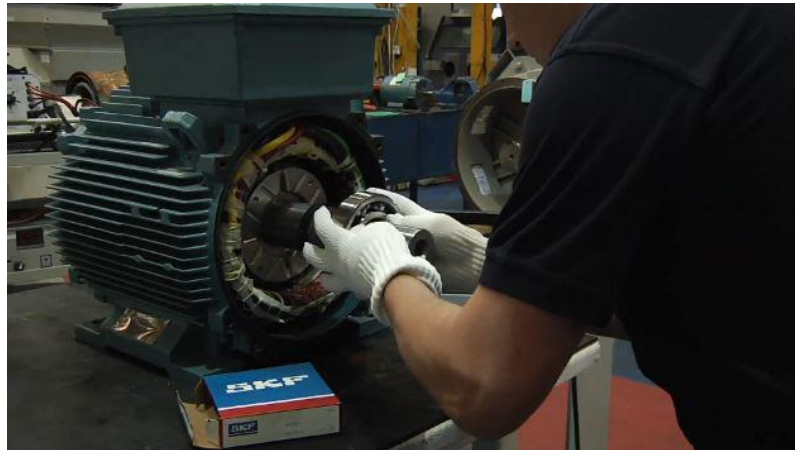
Figure 41: Correct bearing fitting methods
