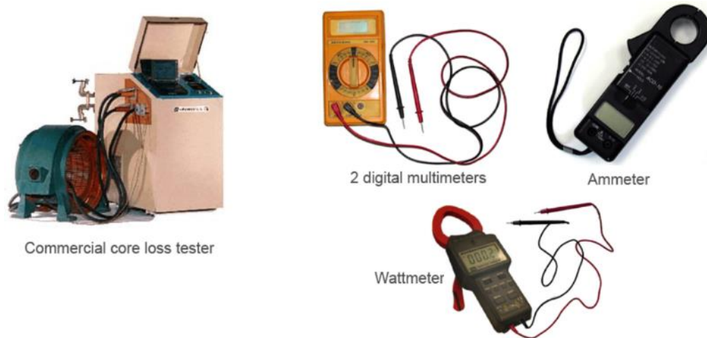
Figure 49: Key equipment and tools used for loss testing
