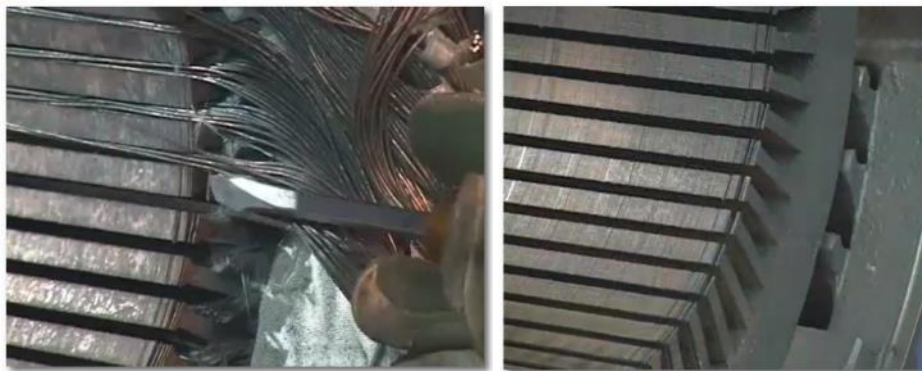
Figure 20: Supporting lamination teeth with a screw driver (left) and a loose stator lamination (right)
