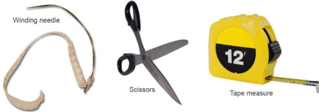
Figure 32: Tools used for lacing motor windings
